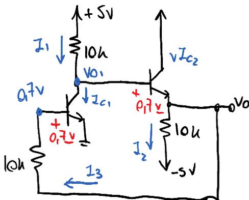
$$\cdot V_{01} = V_0 + 0,7V \quad ; \quad I_3 = I_{B1} = \frac{I_{C1}}{\beta}$$
