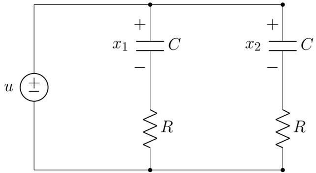
$$\begin{cases} u = x_1 + i_C R = x_1 + RC\dot{x}_1 \\ u = x_2 + i_C R = x_2 + RC\dot{x}_2 \\ \dot{x} = \begin{bmatrix} -\frac{1}{RC} & 0 \\ 0 & -\frac{1}{RC} \end{bmatrix} x + \begin{bmatrix} \frac{1}{RC} \\ \frac{1}{RC} \end{bmatrix} u \end{cases}$$
