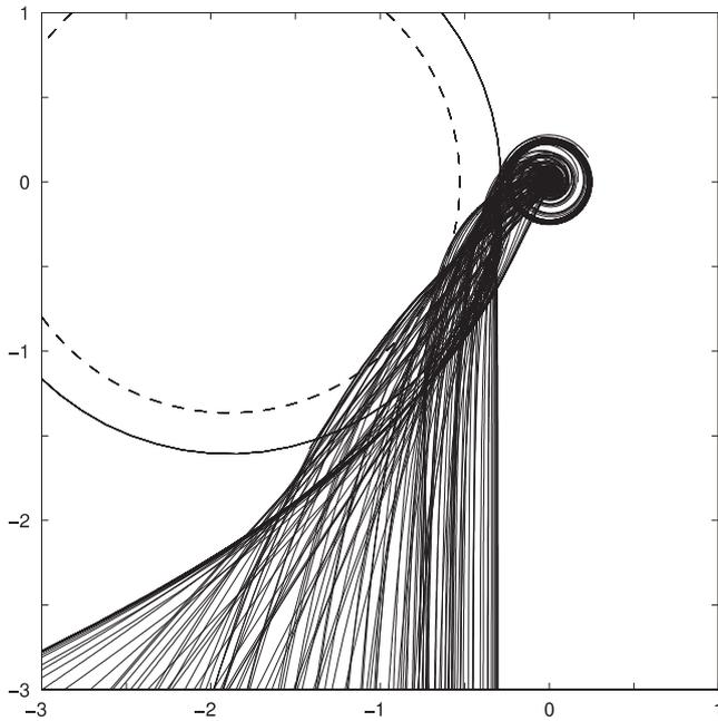
Fig. 9. Nyquist curves of loop transfer functions obtained when PID controllers tuned according to (11) are applied to the test batch (5). The solid circle corresponds  $M = 1.4$ , and the dashed to a circle where  $M$  is increased by 15%.
