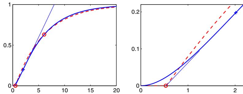
Fig. 3. Step responses of two systems with different dynamics but the same parameters  $K, L$  and  $T$ . The dashed line represents a system with the transfer function  $P_1(s) = e^{-0.54s}/(1 + 5.57s)$  and the full line is the step response of the system  $P_2(s) = 1/((1 + s)(1 + 5s))$ .
