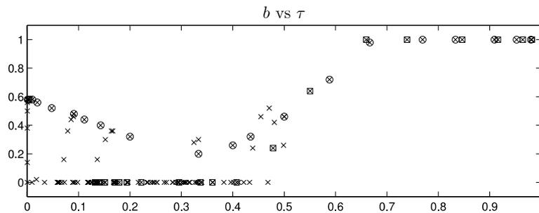
Fig. 10. Set-point weighting as a function of  $\tau$  for the test batch (5). The circles mark parameters obtained from the process  $P_1$ , and the squares mark parameters obtained from the process  $P_2$ .
