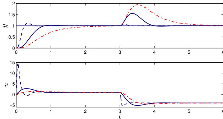
Fig. 14. Responses to a unit step change at time 0 in set point and a load step with amplitude 5 at time 3 for PID controllers designed by AMIGO (full line) and MIGO for PID (dashed line) and PI (dash-dotted line) for a process with the transfer function  $G(s) = 1/((1+s)(1+0.1s)(1+0.01s)(1+0.001s))$ .
