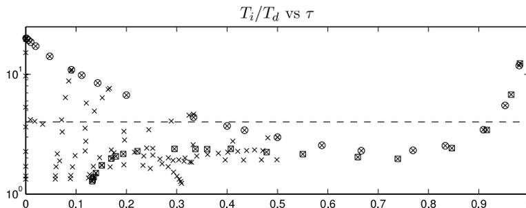
Fig. 6. The ratio between  $T_i$  and  $T_d$  as a function of relative time delay  $\tau$ . The dashed line corresponds to the ratio  $T_i/T_d = 4$ . Process  $P_1$  is marked with circles and process  $P_2$  with squares.
