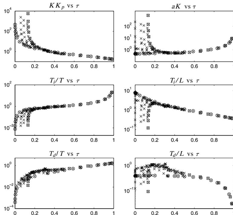
Fig. 2. Normalized PID controller parameters as a function of the normalized time delay  $\tau$ . The controllers for the process  $P_1$  are marked with circles and controllers for  $P_2$  with squares.
