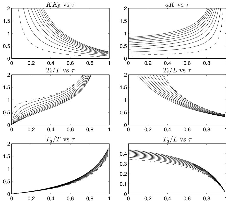
Fig. 12. Controller parameters for the process  $P_1(s)$  as a function of relative time delay  $\tau$  for the tuning parameters  $M = 1.1, 1.2, 1.3, \dots, 2.0$ . The curves for  $M = 1.1$  are dashed.
