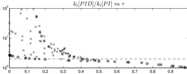
Fig. 5. The ratio of integral gain with PID and PI control as a function of relative time delay  $\tau$ . The dashed line corresponds to the ratio  $k_i[\text{PID}]/k_i[\text{PI}] = 2$ . The controllers for the process  $P_1$  are marked with circles and controllers for  $P_2$  with squares.
