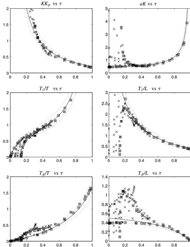
Fig. 8. Normalized controller parameters as a function of normalized time delay  $\tau$ . The solid line corresponds to the tuning rule (11), and the dotted lines indicate 15% parameter variations. The circles mark parameters obtained from the process  $P_1$ , and the squares mark parameters obtained from the process  $P_2$ .
