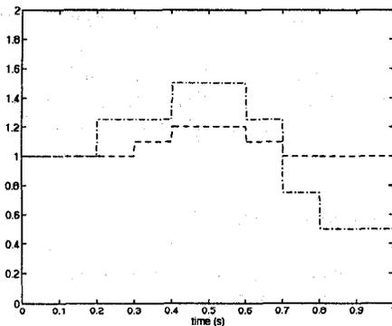
Figure 3: Stator and rotor resistances variation, in p.u.
