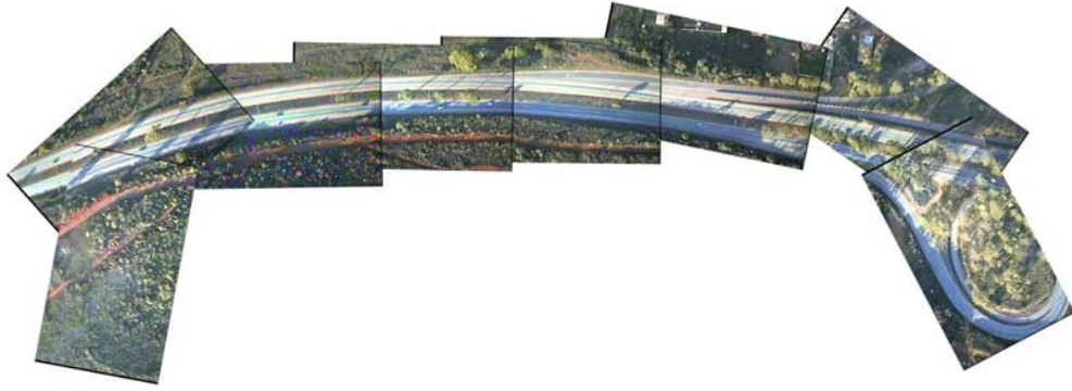
Figure 17. Image mosaicing as the ultimate result of a typical mission accomplished by the hand-launched SUAV.
