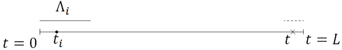
Fig.4.14. A node located at t_i is unable to extend its influence domain \Lambda_i until the point t . But it should, because they are physically close to each other. When an expression that takes the complementary distance into account is employed in the numerical calculation of the shape functions, this problem is solved. The influence domain \Lambda_i now includes point t (the portion of the interval denoted by the dashed line has now been incorporated in \Lambda_i ).
