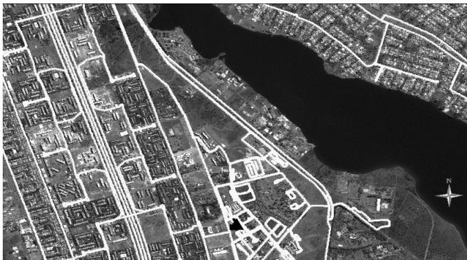
Fig. 2. Measurement tracks (white) and base station (black triangle) shown over an IKONOS satellite image.
