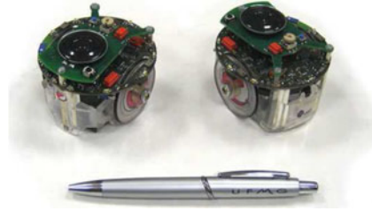
Fig. 10. Two E-Pucks from the VeRLab Swarm. Each E-puck has a 7-cm diameter and is equipped with encoders and bluetooth communication, among other resources.
